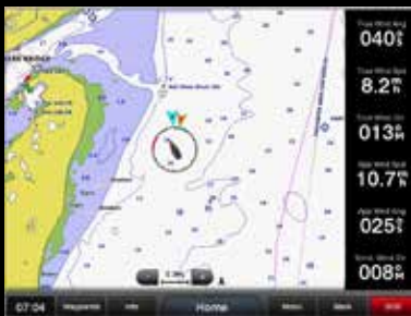
New wind rose Displays true and apparent wind angle at the same time.
