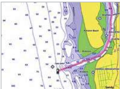
Auto Guidance 3.0 Auto Guidance technology quickly calculates a suggested route using your boat's dimensions and a suggested path to follow.
