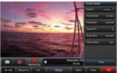
VIRB control bar A control bar can be overlaid on the plotter display to provide quick access to settings and offer a video preview without changing screens.
