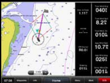
Laylines Shows you on screen when you should make a tack or gybe.
